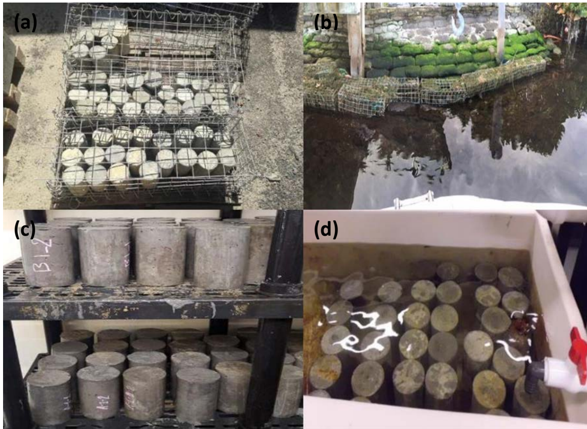
Fig. 13 Different curing regimes (a) subtropical environment; (b) tidal zone; (c) moist curing; (d) immersed in seawater at 60 °C (140 °F).
