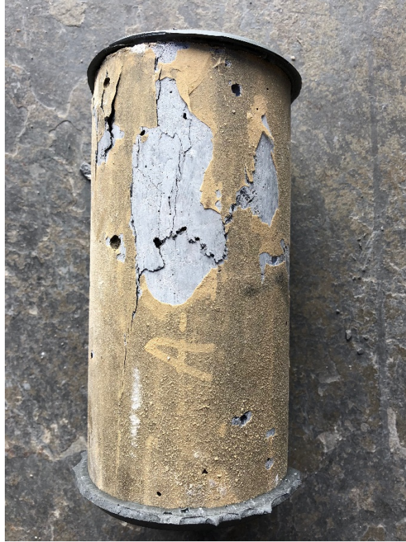
Fig. 19 A layer of leached material covered the surface of a concrete cylinder cast with conventional concrete (Mix A) after immersion in seawater at 60 °C (140 °F) for 24 months.
